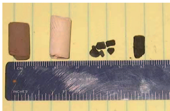
Figure 5. From left to right: Hybrid resorcinol–formaldehyde/iron oxide aerogel; polyisocyanate cross-linked resorcinol–formaldehyde/iron oxide x-aerogel; mesoporous iron aerogel derived from nanosmelting; macroporous iron aerogel derived from nanosmelting of polyisocyanate-cross-linked x-aerogel (image courtesy Nicholas Leventis).
