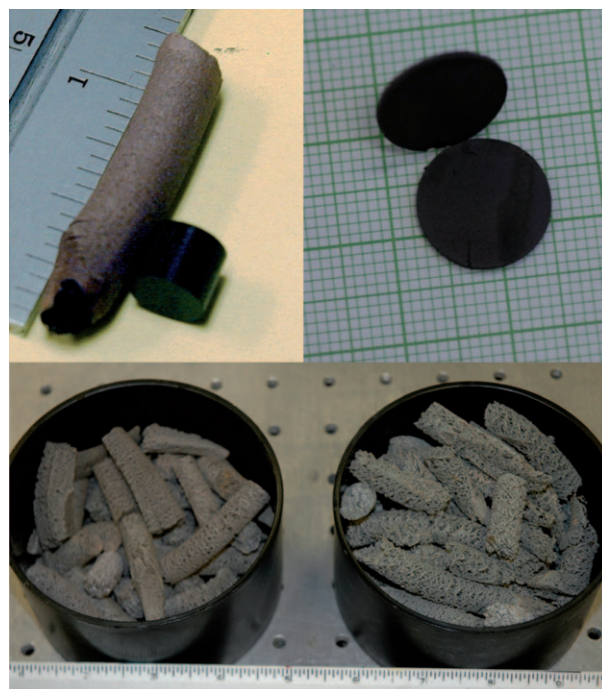
Figure 7. Top left: Fe nanofoam next to an unburnt pellet of FeBTA complex. Top right: Oval- and circle-shaped copper nanofoams. Unlike Fe, Cu nanofoams retain the same shape and size as the unburnt pellet from which they were synthesized. Bottom: Co nanofoams exhibiting porosity ranging from nm to mm.
